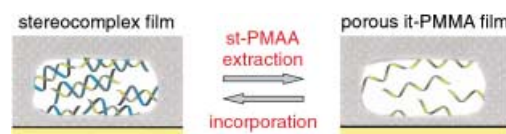
Figure 1. A schematic representation of the selective extraction of st-PMAA from the LbL assembly of it-PMMA and st-PMAA on the basis of stereocomplex formation, and the subsequent incorporation of st-polymers of methacrylic acid or methacrylates.
